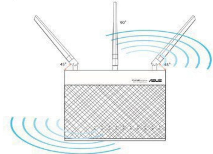
Figure 26: Antennas orientation for best wireless signal
