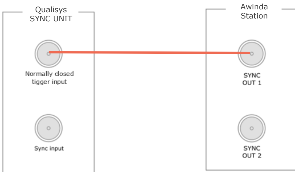
Figure 5 - Connection with BNC-BNC cable scheme to Start and Stop a recording.
