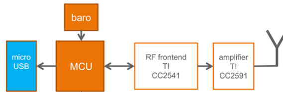
Figure 97: Awinda Dongle ANT block diagram
