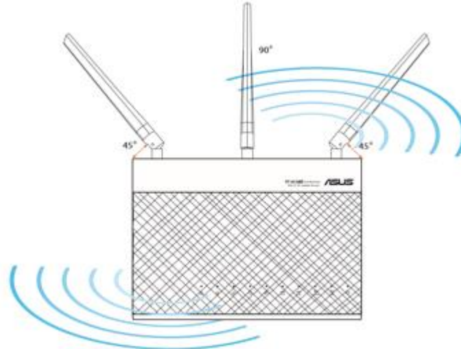
Figure 26: Antennas orientation for best wireless signal
