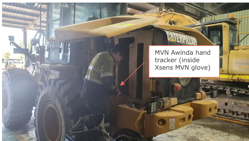
Figure 9: A Diesel Fitter instrumented with full-body 17 sensor Xsens MVN Awinda setup. Note that the sensors can be placed under clothing as occlusion is a non-issue with inertial-based motion capture.
