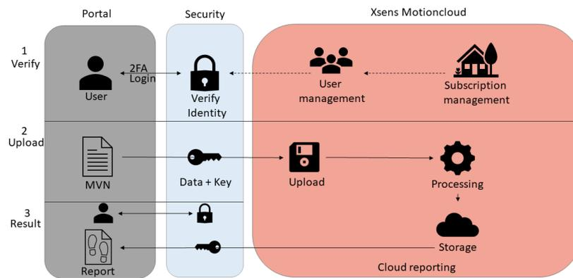
Figure 1: Xsens cloud architecture
