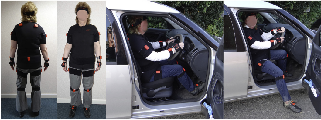
Fig. 1. Magneto-inertial motion capture system attached to a subject – the sensors are the small “matchboxes” attached to the subject.
