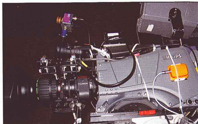
Figure 2. The TV camera with attached inertial sensor, fisheye camera, and lens sensor.
