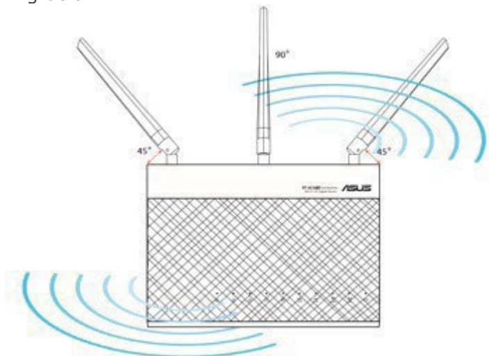
Figure 26: Antennas orientation for best wireless signal
