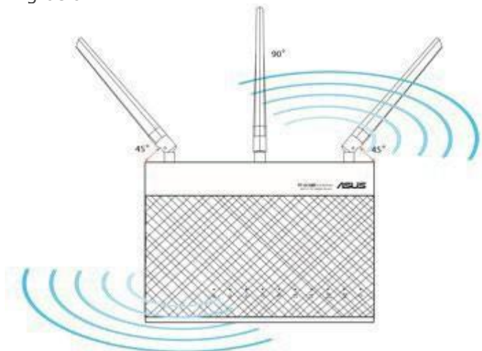
Figure 26: Antennas orientation for best wireless signal
