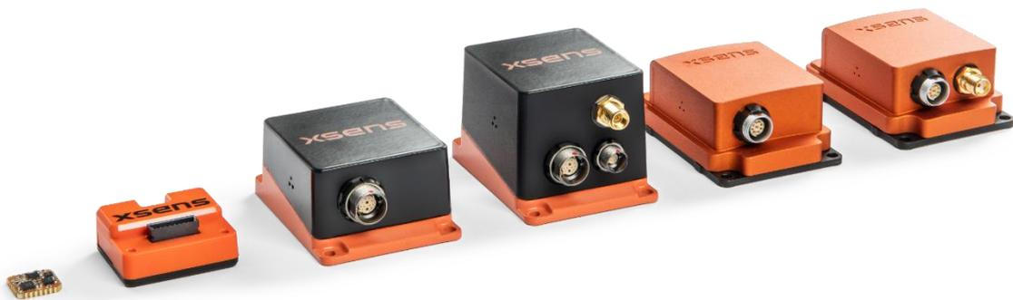
Figure 1: The Xsens MTi series line-up, showing (from left to right) the MTi 1-series, MTi 600-series and MTi 100-series.
